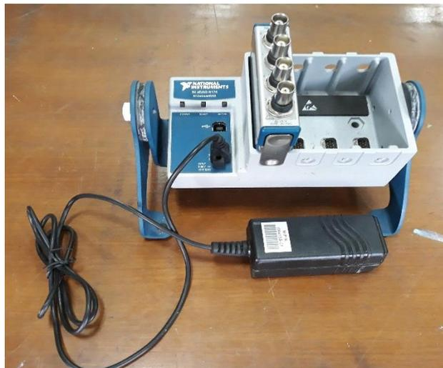
Gambar 3. 13 *Chassis* modul DAQ
