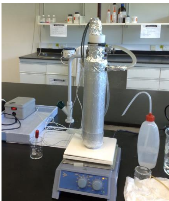
Figure 3. 4 UV/H 2 O 2 oxidation experimental set up.
