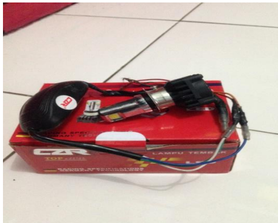
Gambar 3.3 Lampu utama LED CZR (AC & DC 9-30 V, power 40 Watt)
