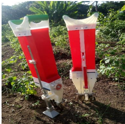
Gambar 2.1 Jenis Tugal Mekanik Alat penanam mekanik tipe dorong. Sumber : https://www.galaxindo.com/uploads/galaxy-catalogue.pdf
