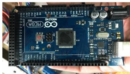
Gambar 2. 10 Arduino Mega 2560
