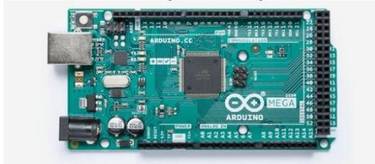
Gambar 2.3. Arduino Mega 2560
