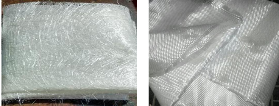
Gambar 2.8 Serat acak dan serat woven roving 200gr
