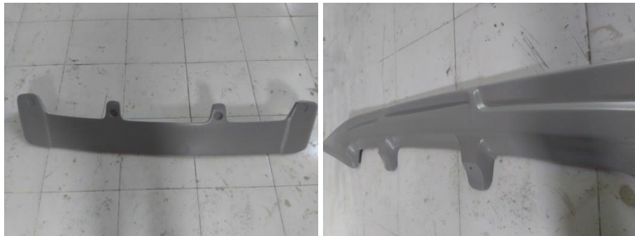
Gambar 4.15 spoiler dicat dasar epoxy
