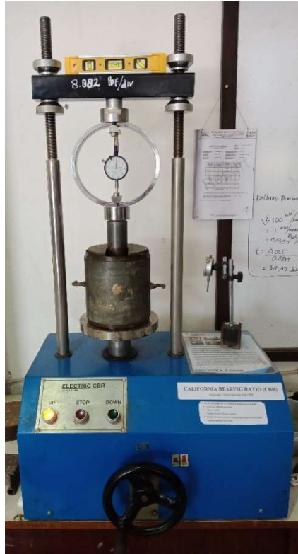
Gambar 3.22. Pengujian Penetrasi CBR ( California Bearing Ratio ) Laboratorium
