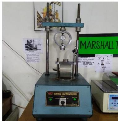
Gambar 3.15 *Marshall electrical machine*
