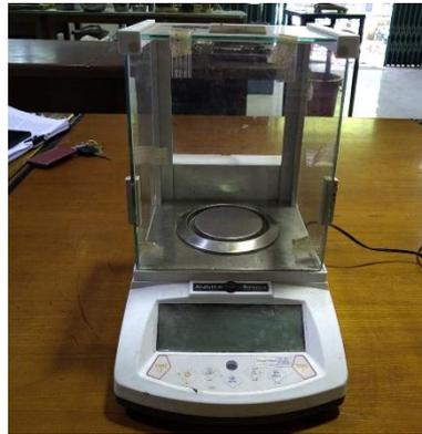
Gambar 3.6 Timbangan *analytical balance*
