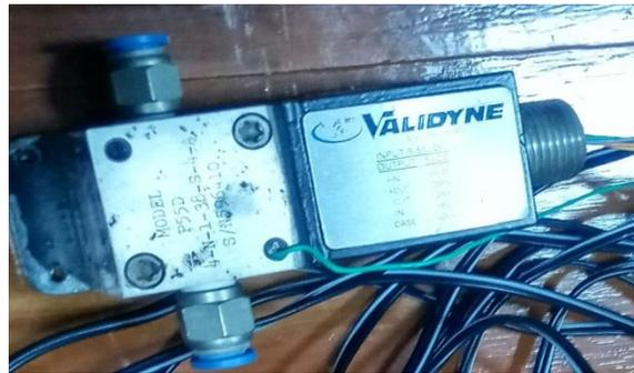
Gambar 3.12. *Pressure transducer*
