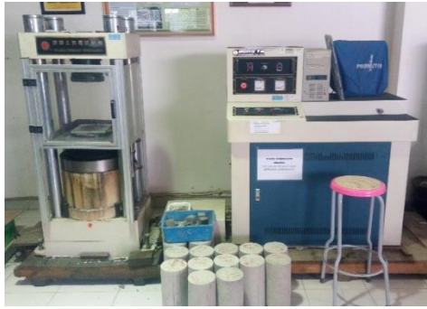
Gambar 3.10 Alat uji beton Concrete Compressive Strength Machine
