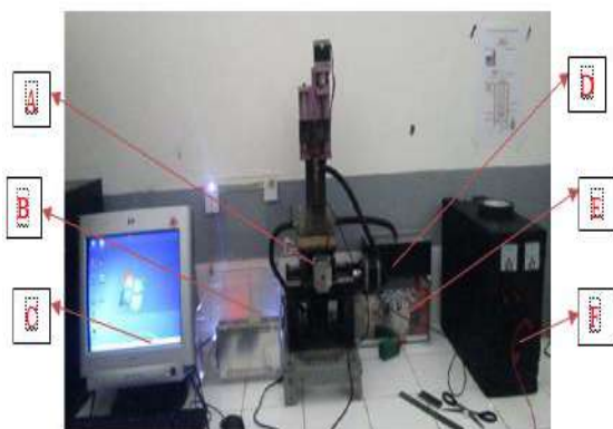
Gambar 1. Konfigurasi mesin ECM, (A) mesin ECM portable, (B) controler motor stepper, (C) computer, (D) filter, (E) reservoir, (F) power supply.
