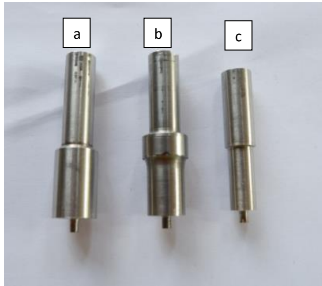
Gambar 3.6 Pin Tool (a). Rasio Shoulder 16/3 mm/mm, (b). Rasio Shoulder 14/3 mm/mm, (c).Rasio Shoulder 10/3 mm/mm.
