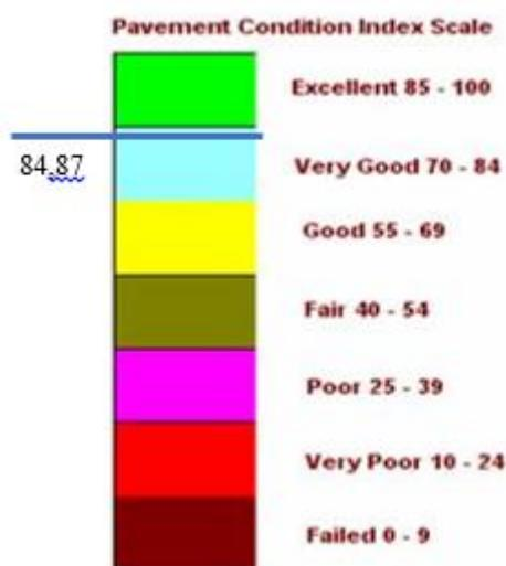
Gambar 18 *Pavement Condition Index Scale*
