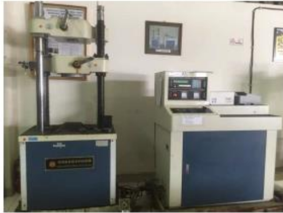
Gambar 3. 10 Alat uji beton Concrete Compressive Strength Test .
