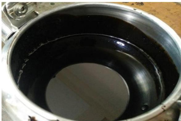
Gambar 3.6 Material aspal penetrasi 60/70
