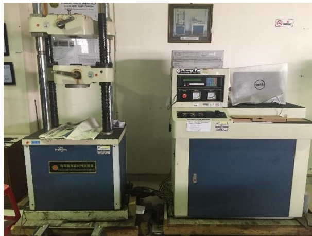
Gambar 3. 6 Flexural Machine Test
