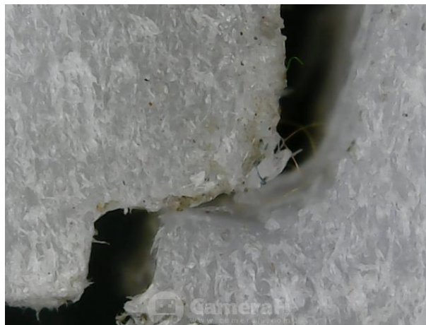
Gambar 4.10 Patahan uji tarik variasi feed rate 10mm/menit
