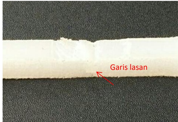
Gambar 4.13 Hasil uji tarik variasi feed rate 20mm/menit
