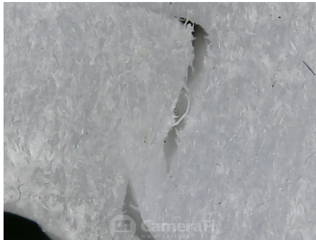
Gambar 4.14 Patahan uji tarik variasi feed rate 20mm/menit
