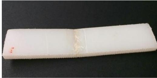
**Gambar 14** Variasi feed rate 10mm/menit uji bending
