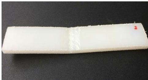
**Gambar 15** Variasi feed rate 14mm/menit uji bending
