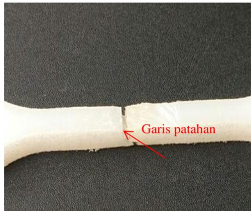
**Gambar 7** Hasil lasan variasi feed rate 10mm/menit
