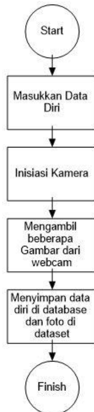
Gambar 4. 6 flowchart system face recognition bagian input data
