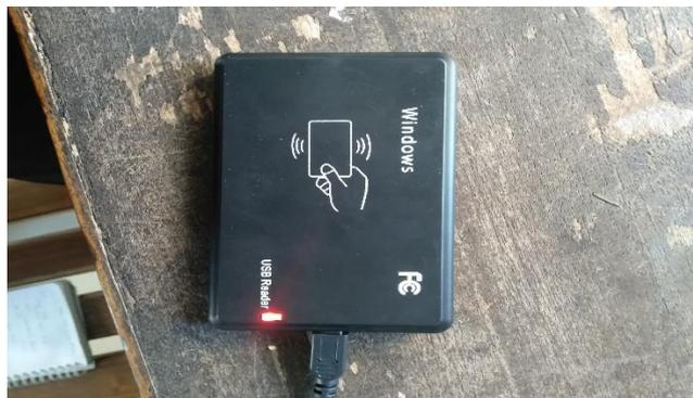
Gambar 4.12 *Reader RFID* (*Radio Frequency Identification*)
