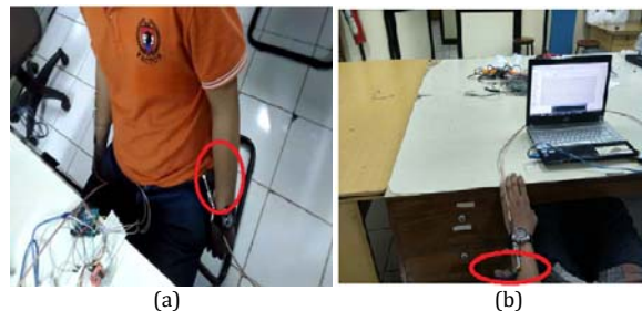
Figure 1. (a) Tx antenna is attached on subject 1; (b) Rx antenna is attached on subject 2.
