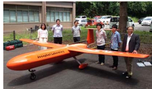
Fig. 4. The 2nd Josaphat Laboratory Experimental Unmanned Aerial Vehicle (JX-2) for microwave sensor ground test
