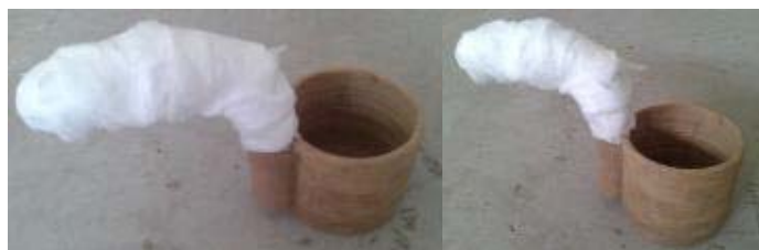
Figure 14, Bamboo component that has been covered with insulating materials
