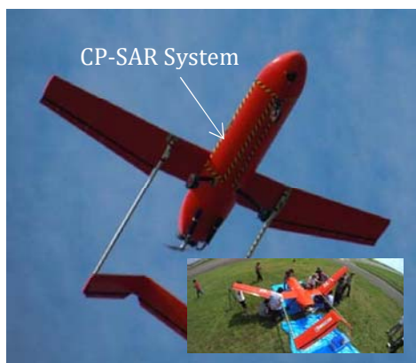
Fig. 3. Flight test of CP-SAR onboard UAV JX-1 at Fujikawa Airport, Japan on 29 August 2013.
