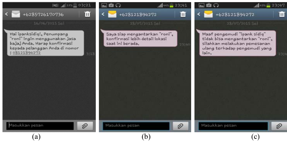
Figure 9. System messaging (a) Passenger call on Driver's phone, (b) Driver confirmation on Passenger's phone, and (c) Driver unable to comply
