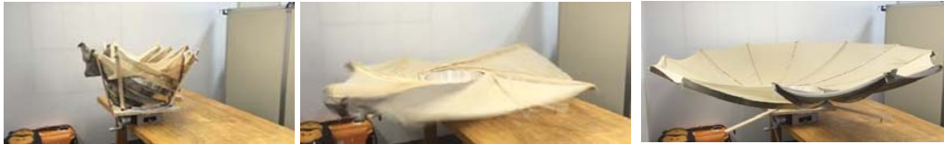
Fig. 7. Deployment experiment of meshed parabolic antenna
