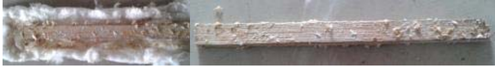
Figure 8. The result of kiln process, \pm 12 mm sodium polyacrylate and ceramic fibre blanket coating layer, bamboo thickness 8 mm.
