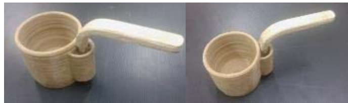
Figure 12. Joining of bamboo component (handle) and clay component
