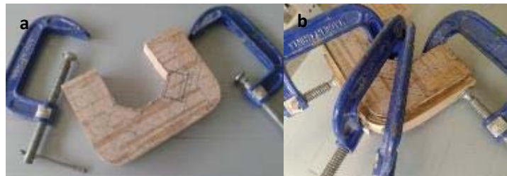
Figure 9. (a) Bamboo laminated bending mold; (b) Cold press bending process
