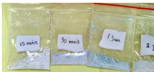
Figure 6. The results of CaO nanoparticles reaction against the gas emissions in PT. Semen Padang
