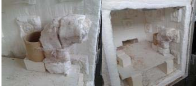
Figure 15. Bamboo and clay component position inside the kiln and ready to burning process
