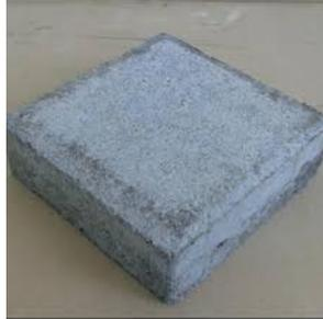
Gambar 2.10 Paving Block Kubus
