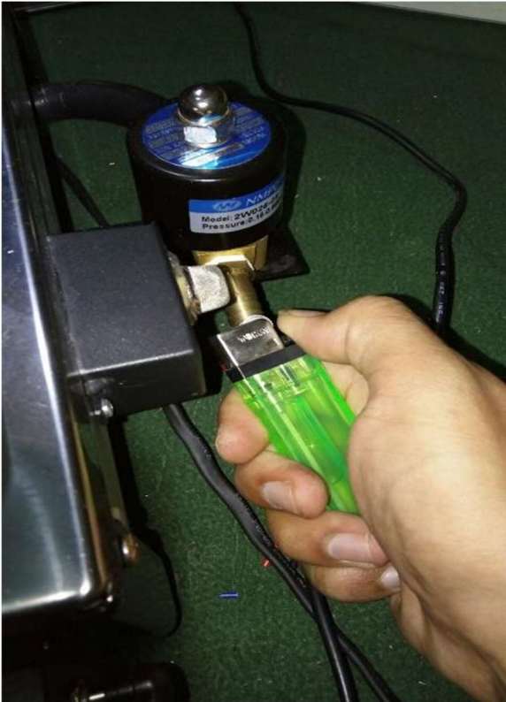
Gambar 4. Uji coba sensor gas
