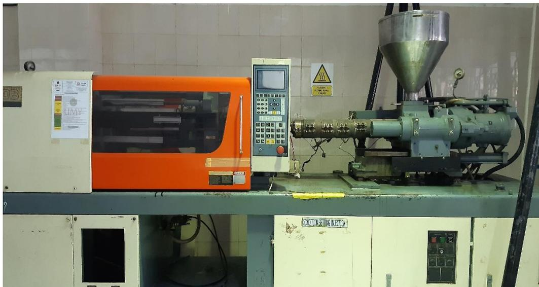
**Gambar 3.2.** Mesin Injection Molding
