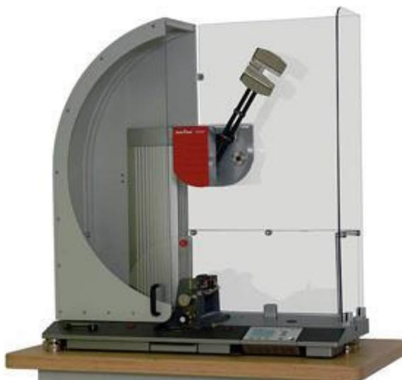
**Gambar 3.4.** Alat Uji Impak Model Charpy
