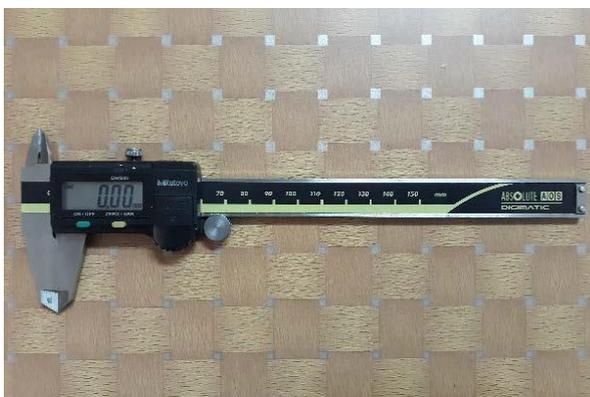
**Gambar 3.7.** Jangka Sorong Model Digital
