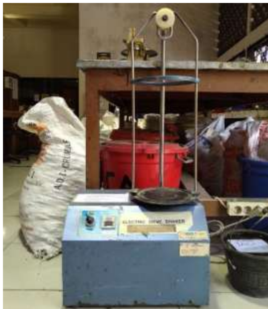
Gambar 3.16 Mesin Sieve Shaker machine
