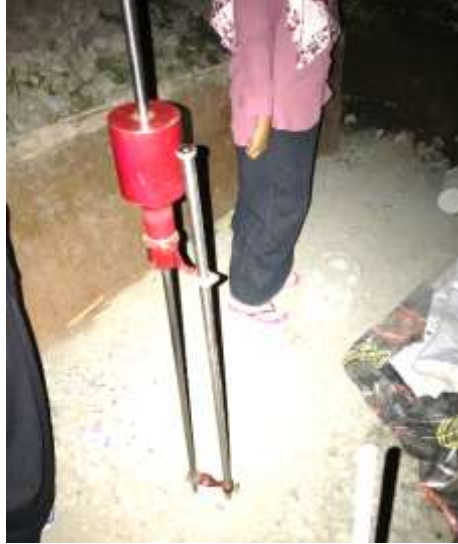
Gambar 3.19 Posisi alat DCP ( Dynamic Cone Penetrometer )
