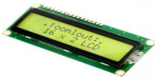
Gambar 2.4 *Liquid Cristal Display (LCD)* [14]
