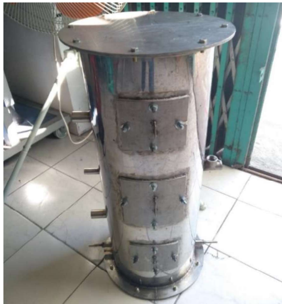
Gambar 3. 6. Tangki solar water heater belum terpasang glasswool dan aluminium.
