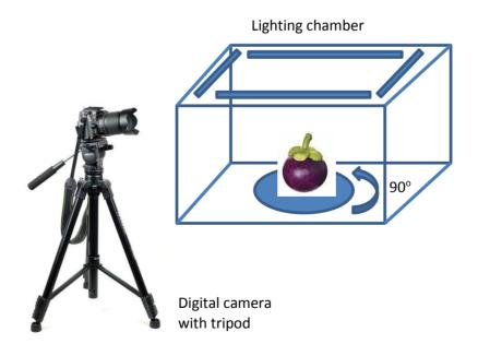
Figure 1: Equipment setup for image acquisition consists of lighting chamber and digital camera with tripod. Mangosteen was rotated 90° to obtained whole surface images.
