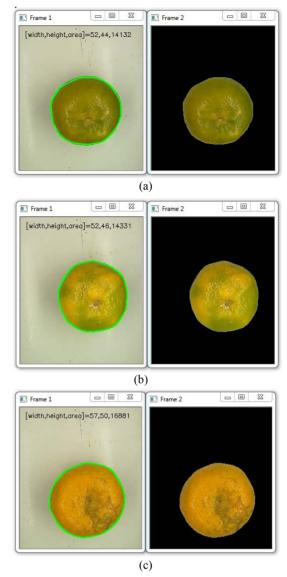
Figure 6. The result of the object selection generates min-max diameter and the area inside the hull polygon of an orange with (a) low ripeness, (b) medium ripeness and (c) high ripeness.
