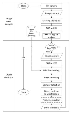
Figure 3. Flowchart of object detection using HSV thresholding and contour detection.
