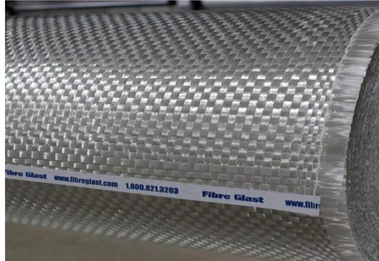
**Gambar 2.4** *Fiberglass woven roving*
