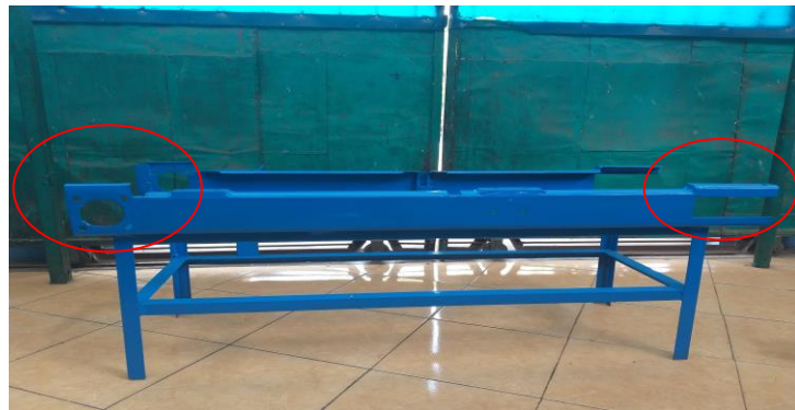
Gambar 4.15 Dudukan bearing dan roller conveyyor
