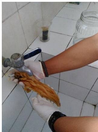
Gambar 3.13. Proses Pencucian Serat Abaca
