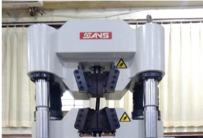
Gambar 3.28. Alat uji tarik Universal Testing Machine (UTM)
