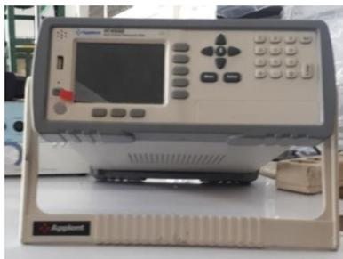
Gambar 3. 8 Applent Temperatur Data logger
