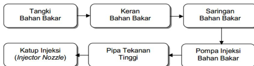
Gambar 2.6 Diagram aliran system bahan bakar
