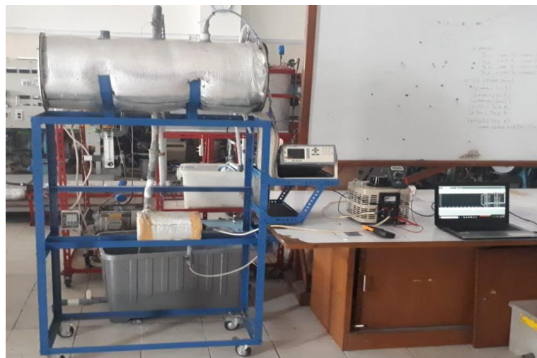
Gambar 3. Tangki Solar Water Heater
