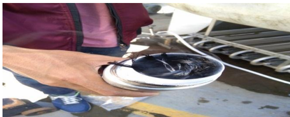
Gambar 3.19 Proses perendaman serat karbon
