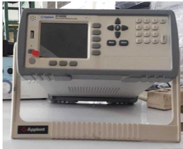
Gambar 3.6 Applent Temperature Data Logger
