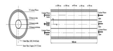
Figure 2: Detail dimension of the test section
