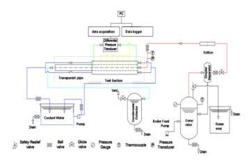
Figure 1: Schematic installation of the experimental apparatus.
