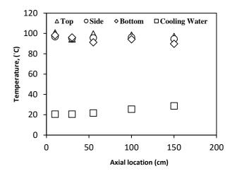
**Figure 10:** Typical Temperature profiles on the cross-section test pipe (mst = 5,9 x 10-3 kg/s, mco = 4,23 x 10-1 kg/s)
