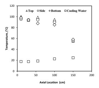
**Figure 7:** Typical of Temperature profiles on the cross-section pipe test (mst= 1.4 x 10-3 kg/s, mco = 4.23 x 10-1 kg/s)
