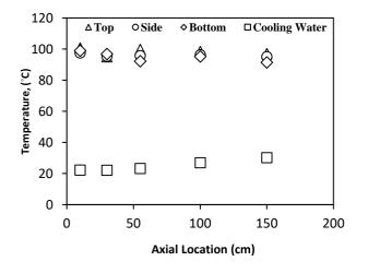
**Figure 12:** Temperature profiles on the cross-section test pipe (mst= 1.1 x 10-2 kg/s, mco = 4.23 x 10-1 kg/s)
