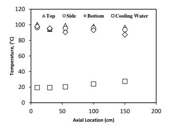
**Figure 9:** Typical of Temperature profiles on the cross-section pipe test (mst= 2.7 x 10-3 kg/s, mco = 4.23 x 10-1 kg/s)
