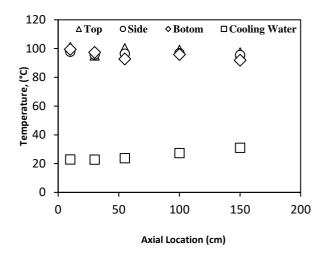
**Figure 13:** Temperature profiles on the cross-secti on test pipe (mst= 1.9 x 10-2 kg/s, mco= 4.23 x 10-1 kg/s)
