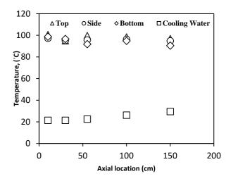
**Figure 11:** Temperature profiles on the cross-section test pipe (mst= 8.9 x 10-3 kg/s, mco = 4.23 x 10-1 kg/s)
