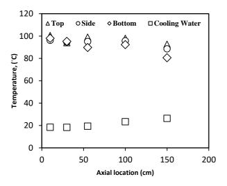
**Figure 8:** Temperature profiles on the cross-section of test pipe (mst= 1.6 x 10-3 kg/s, mco = 4.23 x 10-1 kg/s)
