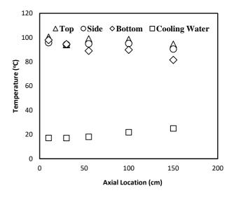
**Figure 6:** Temperature profiles on the cross-section pipe test (mst = 6.9 x 10-4kg/s, mco = 4.23 x 10-1 kg/s)
