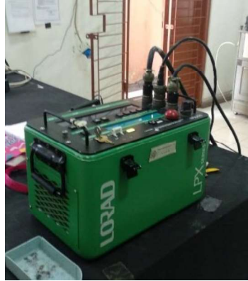
Gambar 3.8 X-ray control console Lorad LPX200
