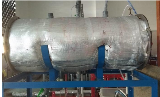
Gambar 3.3 Tangki Solar Water Heater
