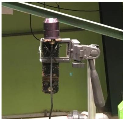
Gambar 3. 5. *Pyranometer*
