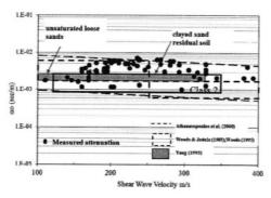
Fig.5. Attenuation factor from this study compared to the attenuation curve from other researchers.
