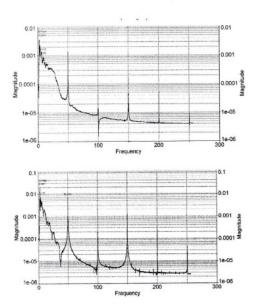
Fig. 2. PSD from SASW measurement on 8 m receiver spacing.
