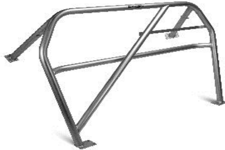
Gambar 2.10 Desain Rollbar 4 Titik ( tf-works.com)
