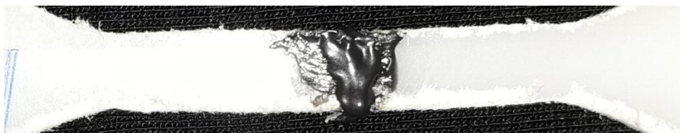
Gambar 4.4 Hasil Sambungan Lem Plastic Steel Epoxy .
