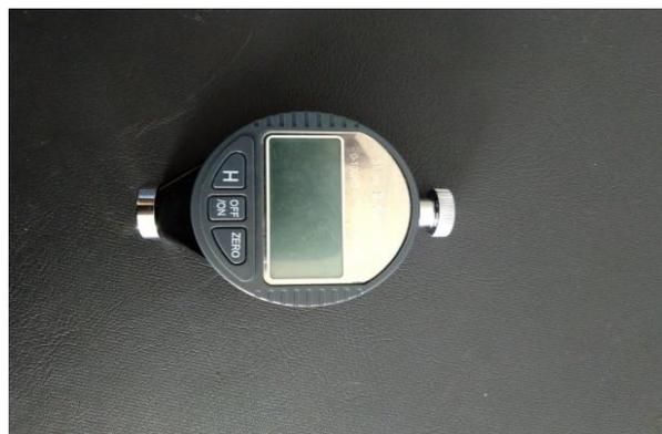
**Gambar 3. 4** Alat Uji Kekerasan *Shore Durometer*
