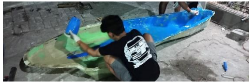
Gambar 9. Proses laminasi bodi
