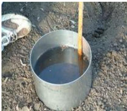
Gambar 4.3 Single ring infiltrometer
