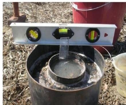
Gambar 4.4 double ring infiltrometer
