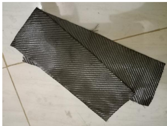
Gambar 3.12 Serat carbon aramid .
